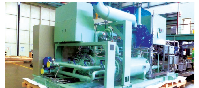
Instrument Air Compressor for Combined Cycle Power Plant
