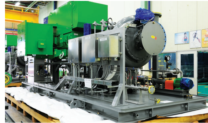
Process Air Blower for Sulfur Recovery Unit
