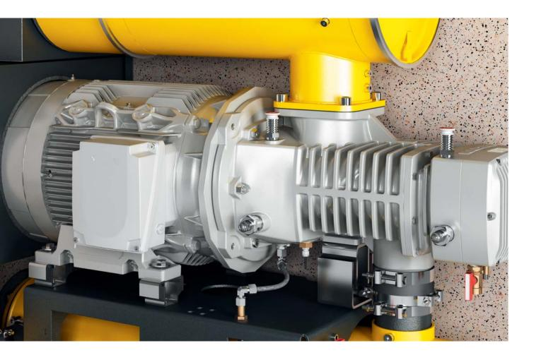
In DBS series screw blowers, power is transferred from the motor to the blower airend via an integrated gear transmission. Following detailed examination in the KAESER Research and Development Centres, this was found to be the most effective transmission solution for the speeds in this power and size class with regards to efficiency, dependability and durability.
