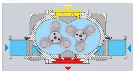
If vacuum (yellow) occurs between the rotor and the casing ambient air (blue) enters the blower block via so-called pre-inlet channels as the rotors continue to turn. The two volume flows subsequently combine and the arising compression heat is dissipated throughout a much larger volume of trapped air. This approach therefore achieves the same discharge temperatures that are produced by normal blower blocks.
