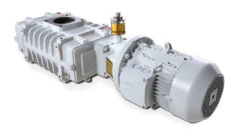
When producing fine vacuum in combination with a corresponding backing pump, the WVC significanItly increases pump suction capacity and vacuum performance. The use of a frequency converter is particularly beneficial, as the converter enables simultaneous activation of rotary vacuum and backing pumps at atmospheric pressure, thereby significantly reducing pumping time.
